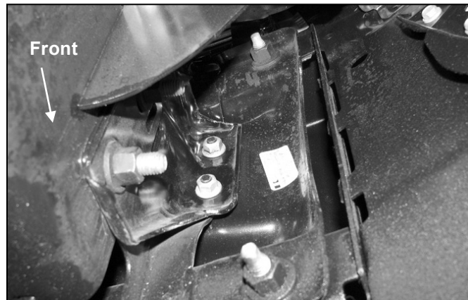
(Fig 2) Tow hook mounting hardware from behind the passenger/right side of the bumper
